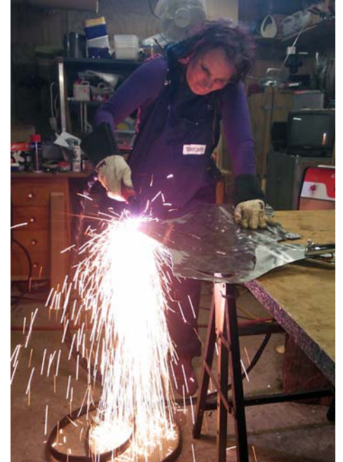
• Sparks fly as Pauline uses the plasma cutter to create her artwork
